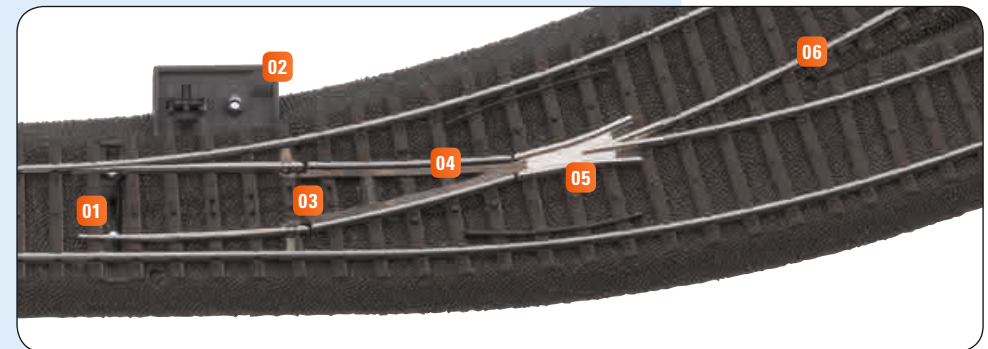
01 Separately mounted, cast switch rails 02 Prototypical built-up roadbed area at the location for the switch linkage 03 Continuous electrical contacts from the switch rails to the frog 04 Intermediate rails made of shaped material 05 Inset metal frog 06 Turnout curve as a 30° section of a circle, radius 360 mm / 14-3/16"
